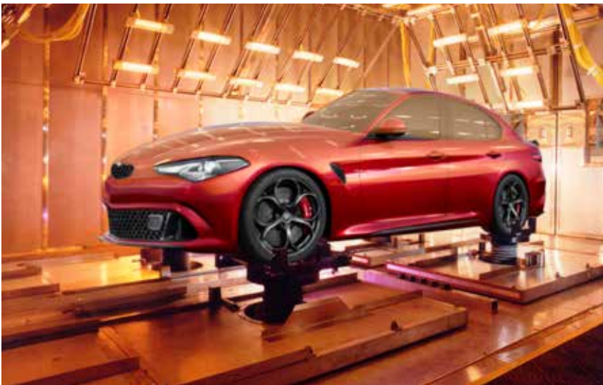
Four post road simulator with temperature, humidity, vibration and solar simulation.
